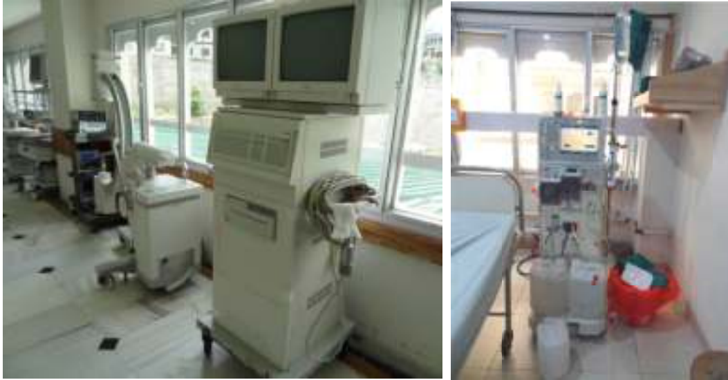
Figure 38. Mobile equipment used in OTs stored without tethers in hallway (left); tall, narrow dialysis equipment (right)
