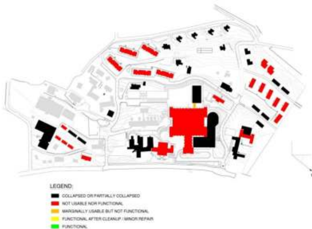
Figure 50. Likely performance of hospital buildings in M8.6 hypothetical scenario earthquake
